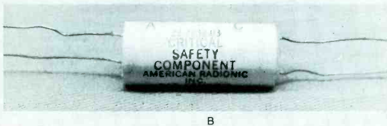
Fig. 13 In the 1975 models 17FC45 and 19FC45, the many individual capacitors which in previous models were connected in parallel between collector and emitter of Q202, are replaced by one special capacitor. (A) The circuit shows the capacitor has four leads, so the circuit goes through the capacitor. An open capacitor (or one removed) completely eliminates the sweep. Notice that the capacitor and the flyback transformer are not the same for the 17" and 19" models. (B) In appearance, the capacitor resembles conventional ones, except for the extra two leads.
